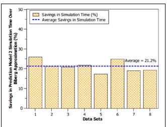
Fig. 5. Savings in prediction computational time of proposed model 2 over Biberg (1999); plot of t\_savings for experimental cases in Table 1.
