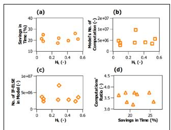
Fig. 6. Correlation plots between liquid holdup and (a) savings in computational time of proposed model 2 with respect to Biberg's approximation (b) number of computations in proposed model 2 and (c) number of IF-ELSE statements in proposed model 2. (d) Correlation plot of computation ratio and savings in computational time. Computation ratio is the ratio of number of computations in Biberg's approximation to number of computations in proposed model 2.
