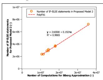
Fig. 7. Number of IF-ELSE statements in Proposed Model 2 is compared with number of computations for Biberg's approximation; data are presented for fixed location in pipeline where flow variation is observed.
